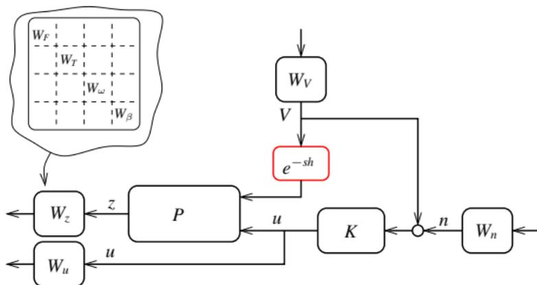
Deviations of wind speed  $V$  = disturbances measured with noise  $n$
