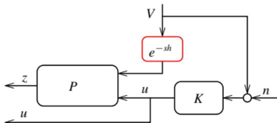
Deviations of wind speed  $V =$  disturbances measured with noise  $n$
