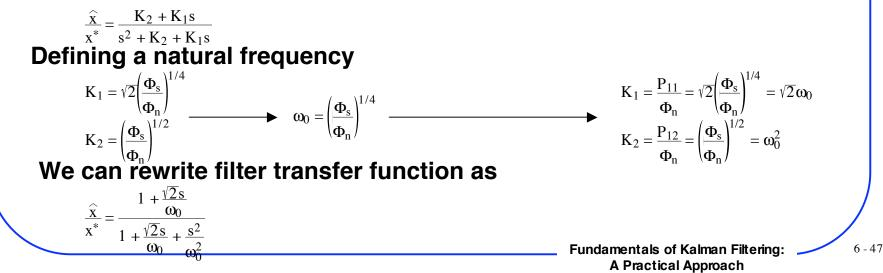
Filter Natural Frequency Increases as the Ratio of the Process to Measurement Noise Spectral Densities Increases
