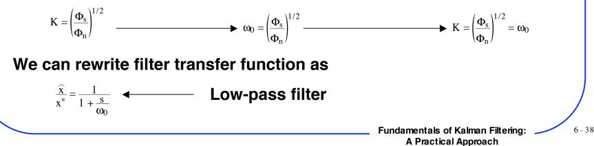
Zeroth-Order Continuous Polynomial Kalman Filter's Natural Frequency Increases as the Ratio of Process to Measurement Noise Increases
