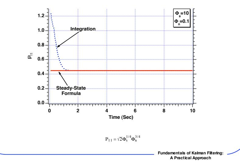
Steady-State Formula for Second Diagonal Element of Covariance Matrix is Accurate for Continuous First-Order Polynomial Kalman Filter
