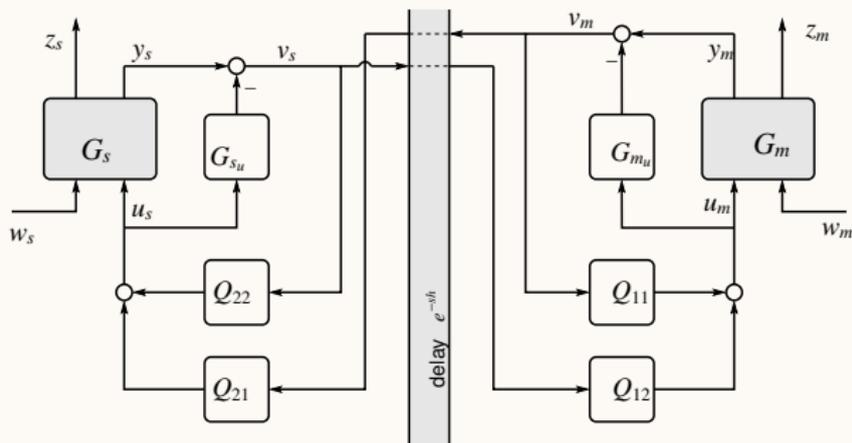
Communication is based on  $v_m$  and  $v_s$  signals
