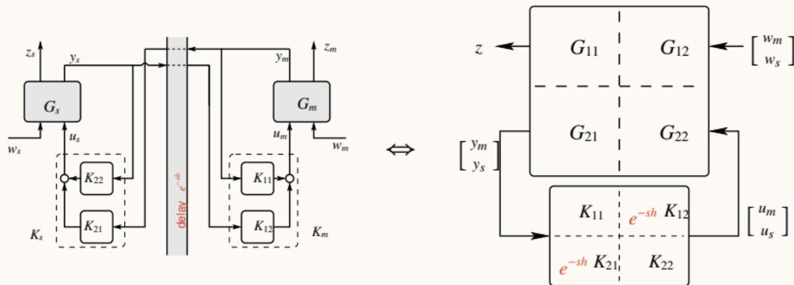
Information constraints  $\Rightarrow$  constraints on controller structure (distributed control)
