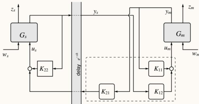
Controller for the remote site can be designed separately
