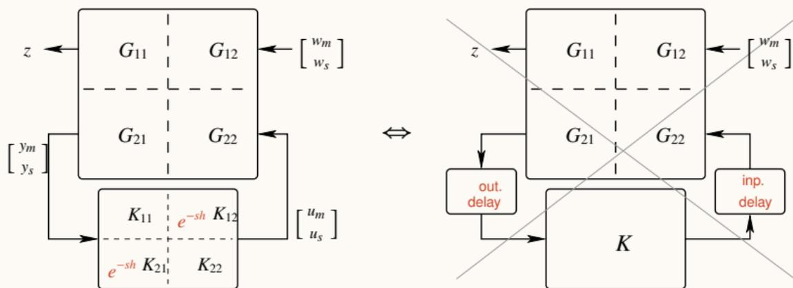
Delays can not be extracted  $\Rightarrow$  **Distributed control problem**
