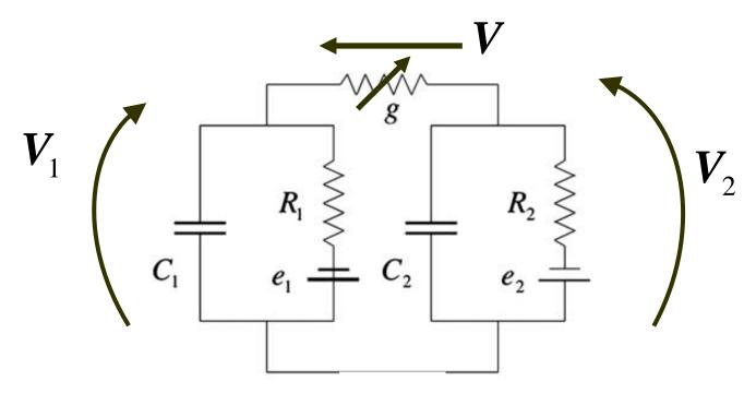
$$C_1 \dot{V}_1 = -(1 / R_1)(V_1 - e_1) - (V_1 - V_2) g(\mathbf{x}),$$
