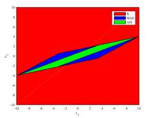
X - State constraints polytope, MAS - Corresponding maximal admissible set using the standard iterative algorithm [see refs.], AS1 - Polyhedral admissible set computed with the algorithm.
