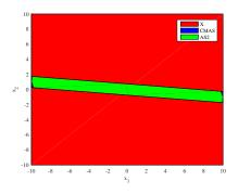
X - State constraints polytope, CMAS - Convex hull of maximal admissible sets using standard iterative algorithm [see refs.] for each of the controllers, AS2 - Polyhedral robust controlled invariant set computed with the new algorithm.
