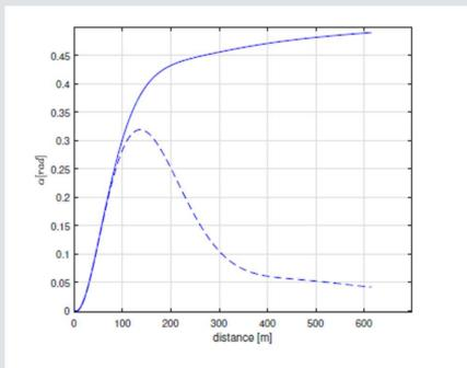
$5^{th}$  scenario, thrust misalignment PD (solid) ; PID (dashed)
